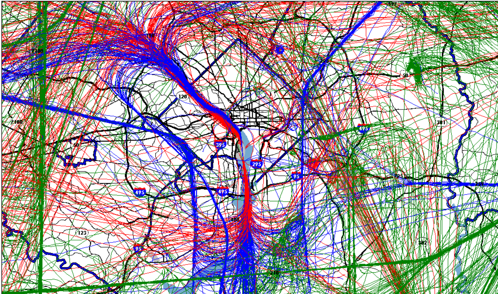
Figure 2 – Typical mixed flow operations for a 24 hour day at Ronald Reagan National Airport. Arrivals are in Blue (447 tracks) , departures are in Red (454 tracks) , and overflights are in Green (1800 tracks) .
